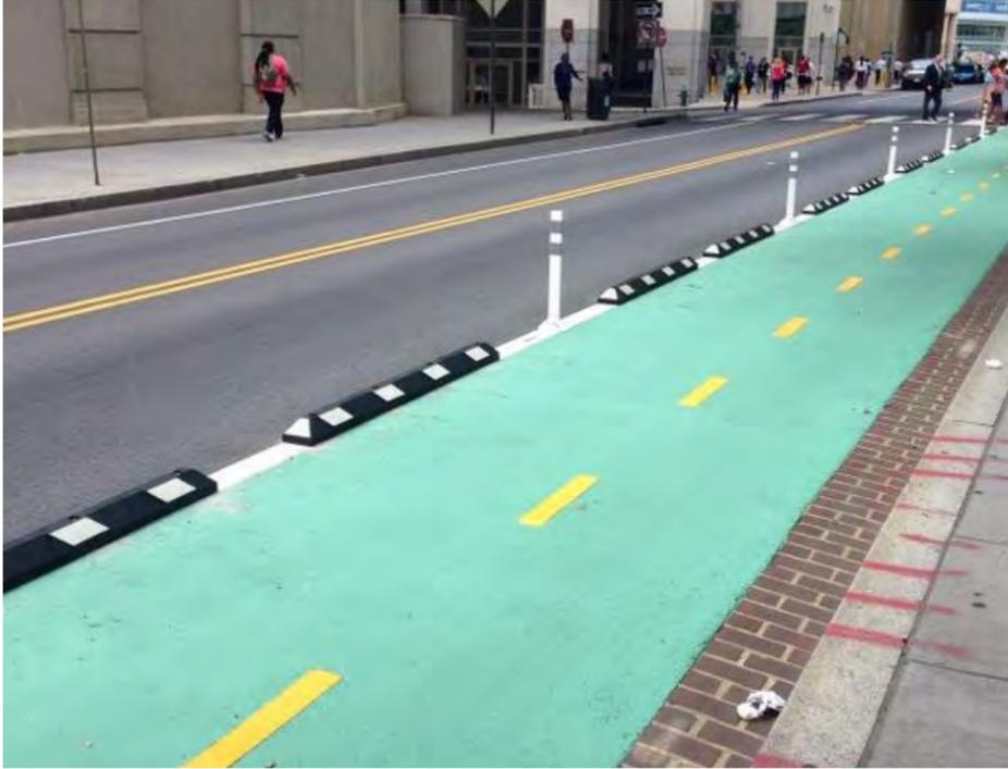
Paint, rubber curbs & flexible bollards (1st St, Washington DC)
